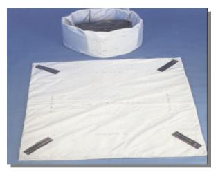
Should the bomb explode, the Safety Circle helps to direct the force of the bomb's explosion upwards then the Bomb Blanket flexes and contains most of the bomb fragments. Two or more Safety Circles can be used together to contain larger bomb devices.
